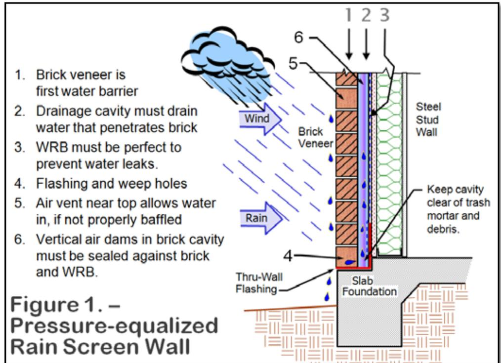
2. The WRB will likely have some holes in it. No construction material is perfect and installation methods are never perfect. The best we can hope for is to provide a nearly continuous air barrier around the building envelope. But where that fails, warm, moist air can get in or out. And many buildings have negative pressure inside that can draw in water vapor, or even liquid water. Adding vents at the top can allow liquid water to enter these holes, not just water vapor.
