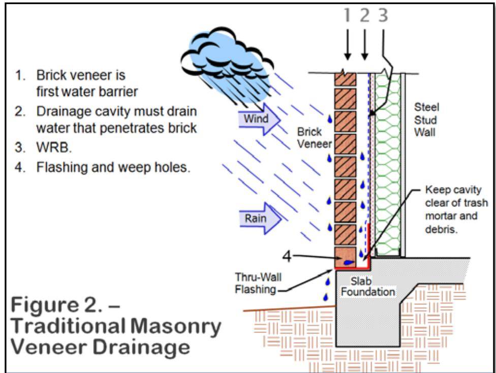
Figure 2. – Traditional Masonry Veneer Drainage
