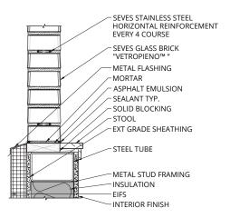
(VP-330) SILL - VETROPIENO™ in Metal Stud **Wall with Synthetic Plaster Finish**
