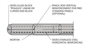
(Q-454) VERTICAL REINFORCEMENT - Glass **End Block Linear Free Standing Wall**
