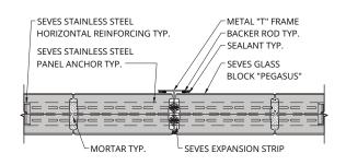
(Q-451) VERTICAL STIFFENER - "T" Intermediate **Vertical Support in Multiple Panels**
