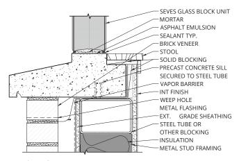
(PD-131) SILL - Glass Block in Metal Stud Wall with Brick Veneer
