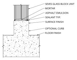
(PD-132) SILL - Glass Block at Concrete Floor Slat with Curb
