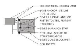
(PD-122) JAMB - Hollow Metal Door Frame at Glass Block
