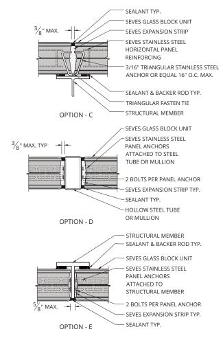
(PD-150) STIFFENERS - Intermediate Support in Multiple Horizontal Panels
