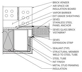
(VB-221) JAMB - VISTABRIK® in Metal Stud Wall with Brick Veneer
