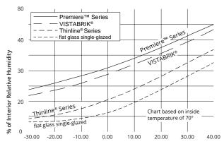
Example: At relative humidity of 40%, an outside temperature of approximately -3°F will cause condensation on Premiere™ Series Glass Block or approximately 3°F above zero on Thinline® Series Glass Block. Under the same conditions, condensation will form on a single-glazed flat glass window at 34°F above zero.
