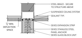
(PD-114) HEAD - Glass Block at Suspended Ceiling
