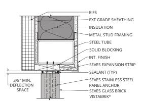
(VB-210) HEAD - VISTABRIK® in Metal Stud with Synthetic Plaster
