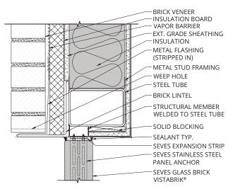
(VB-211) HEAD - VISTABRIK® in Metal Stud Wall with Brick Veneer
