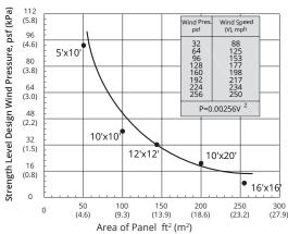
In 2010, ASCE 7 changed from Wind Loads to Strength Level Wind Pressure. The chart above now reflects this change. The new Safety Factor is now 1.7 for all masonry installed glass block panels for further information, please contact Seves Technical Department at 440-672-6257 or email technicalUS@sevesglassblock.com
