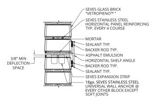
(VP-350) HORIZONTAL STIFFENER - VETROPIENO™ **Intermediate Horizontal Support in Multiple Vertical Panels**
