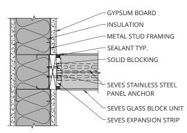
(PD-123) JAMB - Glass Block Perpendicular to Partition
