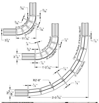
4" AllBend™ Block, Minimum Radius for **Column Construction**
