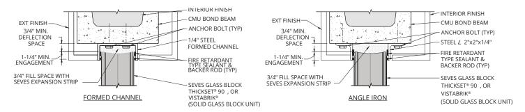
(FR-010) HEAD - 90 Min Fire Rated Glass Block at CMU/Bond Beam
