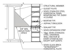
(VP-350) HORIZONTAL STIFFENER - VETROPIENO™ **Structural Horizontal Support in Multiple Panels**
