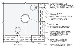
(VP-350) VERTICAL STIFFENER - VETROPIENO™ **Triangular Anchoring at Corner**
