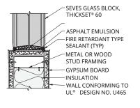
(FR-131) SILL - 45 & 60 Min Fire Rated **Glass Block in Metal Stud Wall**
