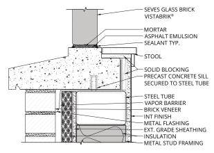
(VB-231) SILL - VISTABRIK® in Metal Stud Wall with Brick Veneer
