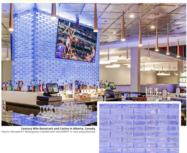
VetroKWiK™ is a snap-together solution for installation of Vetropieno™ solid glass bricks that utilizes clear polycarbonate and ABS plastic in white or gray. This installation system is a no-mess method that uses precise spacing snap-together modules that replace the need for mortar. The VetroKWiK™ Installation System reduces the time to install Vetropieno™ glass block by approximately 50-75%.
