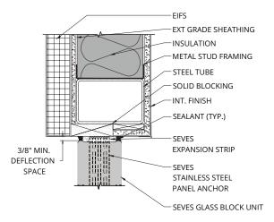
(PD-110) HEAD - Glass Block in Metal Stud Wall With Synthetic Plaster Finish
