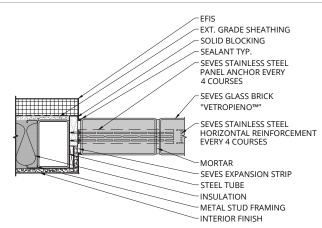
(VP-320) JAMB - VETROPIENO<sup>™</sup> in Metal Stud **Wall with Synthetic Plaster Finish**
