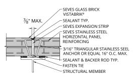
(VB-250) VISTABRIK® Triangle Anchor Intermediate **Support in Multiple Horizontal Panels**
