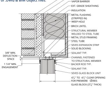
(PD-111) HEAD - Glass Block in Metal Stud Wall With Brick Veneer
